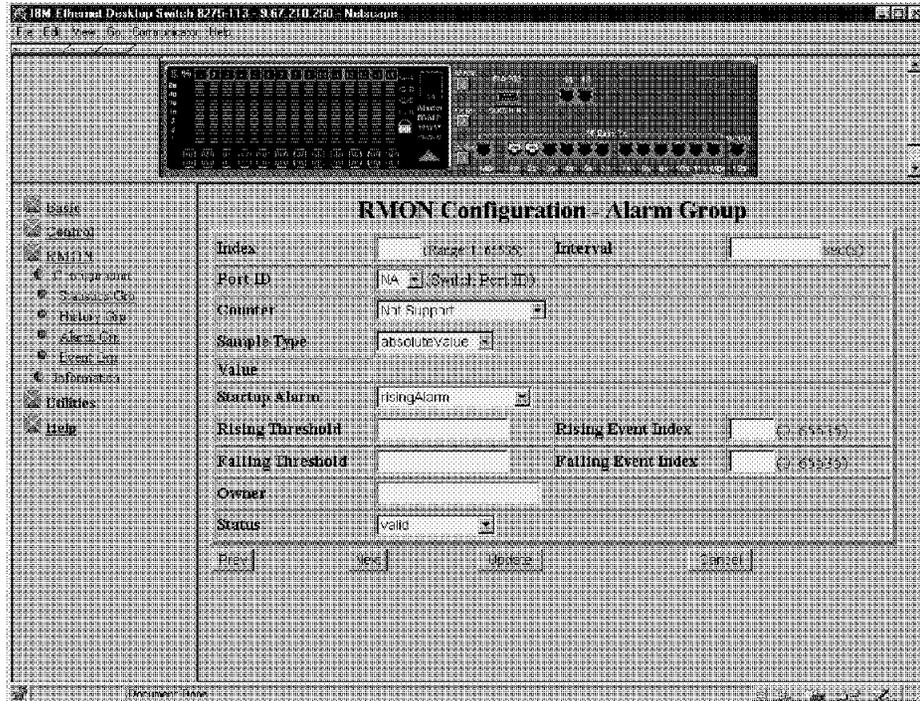
Figura 5-16. Painel RMON Configuration - Alarm Group
